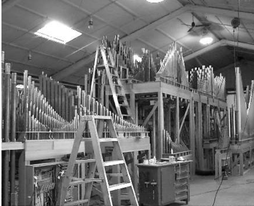
An organ set up for testing at the Wicks Erecting Room. All parts are arranged as they will be in the final installation.
